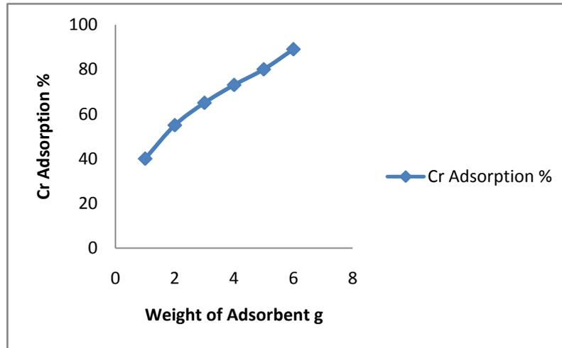
**Fig. 4: Effect of adsorbent dosage on the removal of Cr (VI)**
