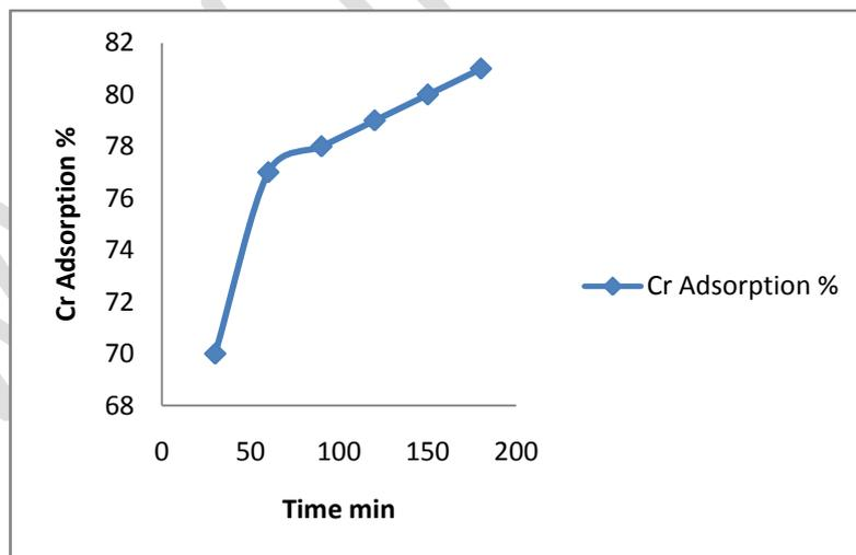
Fig. 3: Effect of contact time on the removal of Cr (VI)
