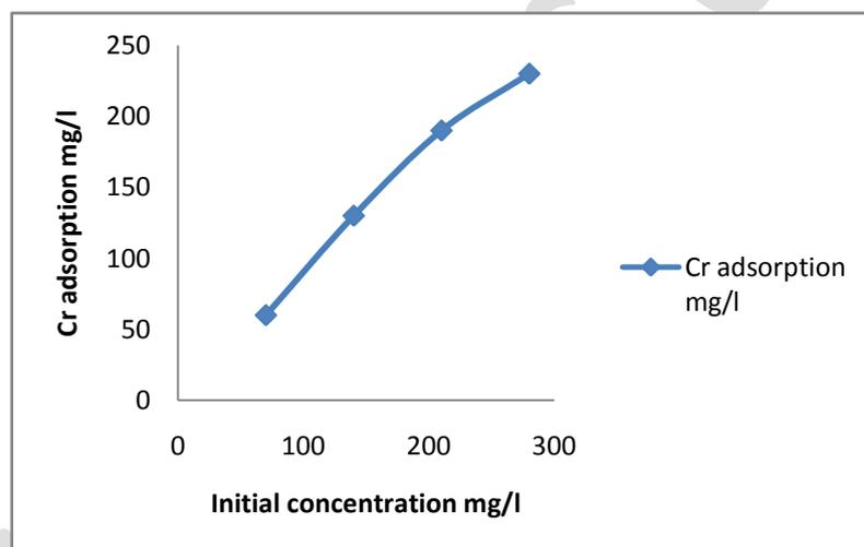
**Fig. 1: Effect of initial concentration on the removal of Cr (VI)**
