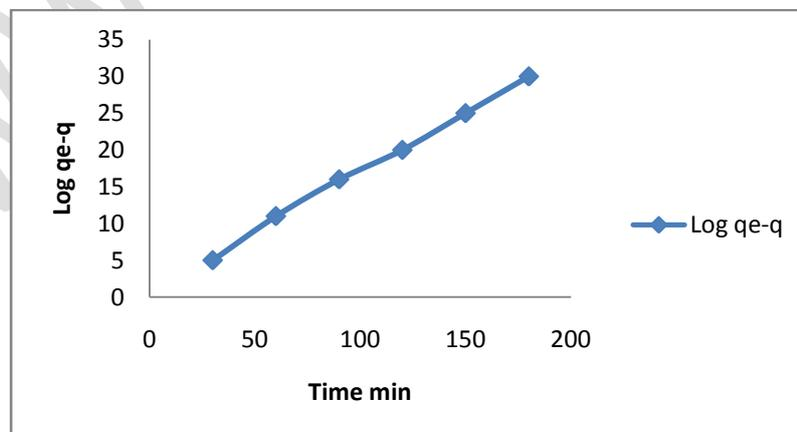
**Fig. 5: Lagergren plot (initial concentration 70 mg/l)**
