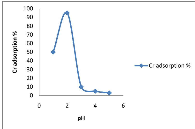
Fig. 2: Effect of pH on the removal of Cr (VI)
