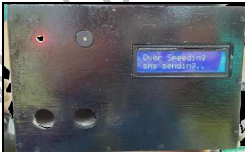
Figure 3. The Android-Based Speed Limit Detector with SMS Support Prototype
